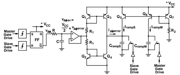
Fig. 6 Implementation of PLL-based control circuit with master-slave interleaving method of two DCM/CCM boundary boost PFC converters that operate with voltage-mode control, when the turn-off instant of the slave converter is adjusted by modifying the slope of the slave's voltage ramp.
