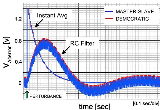
Fig. 12 Simulation of a perturbation of a 400-V/280-W, 127-V<sub>dc</sub> input, interleaved DCM/CCM boundary boost converter with PLL-based closed-loop control for both master-slave and democratic interleaving methods, where the turn-off instant is adjusted by modifying the feedback error voltage, and where the converters operate with voltage-mode control. It should be noted that the waveforms of the master-slave and democratic methods are almost overlapping.
