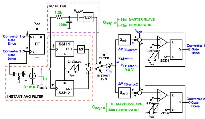
Fig. 10 Simulation subcircuit of a 400-V/280-W, 127 V<sub>dc</sub> input, interleaved DCM/CCM boundary boost converter with PLL-based closed-loop control for both master-slave and democratic interleaving methods, where the turn-off instant is adjusted by modifying the feedback error voltage, and where the converters operate with voltage-mode control.
