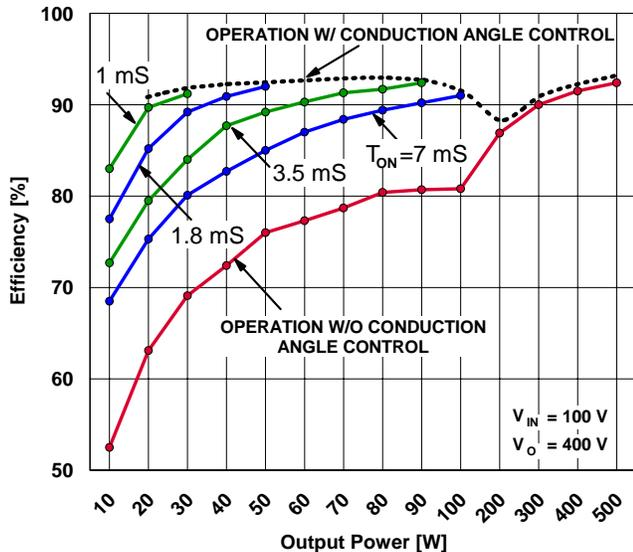
Fig. 13. Measured efficiency of PFC rectifier as functions of output power for different conduction times  $T_{ON}$ . Dashed line represents efficiency that can be obtained by changing (decreasing)  $T_{ON}$  as output power decreases.
