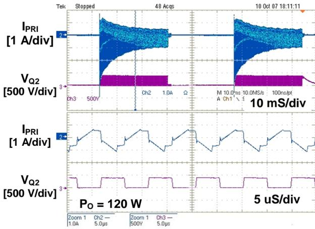
Fig. 9. Measured primary-current  $I_{PR1}$  and switch  $Q_2$  drain-to-source voltage  $V_{Q2}$  waveforms of ZVS full-bridge converter prototype. Time scale for upper two traces is [10 ms/div]. Time scale for bottom two traces is [5 uS/div].
