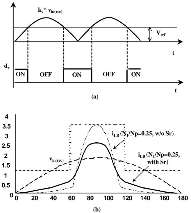
Fig. 8 Improved CCM S<sup>4</sup>-PFC converter with auxiliary switch  $S_r$ :
