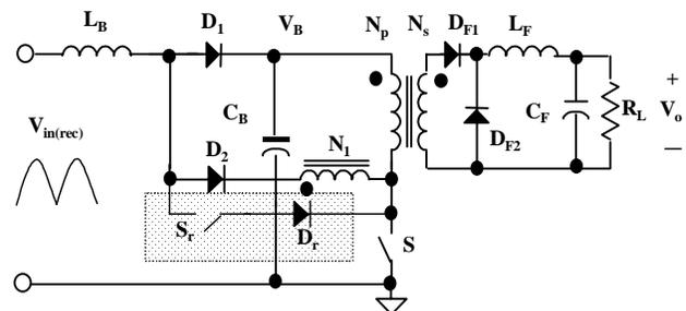
Fig. 18 DCM  $S^4$ -PFC with auxiliary switch  $S_r$ .
