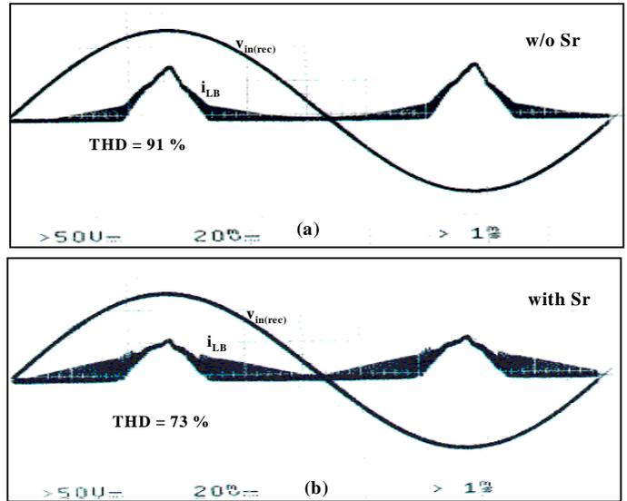
Fig. 9 Measured boost-inductor current  $i_{LB}$  at  $V_{in} = 230 \text{ Vac}$  at full power:
