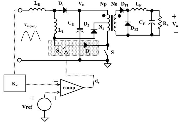
Fig. 7 Conceptual circuit diagram of improved CCM S<sup>4</sup>-PFC converter with auxiliary switch  $S_r$ .
