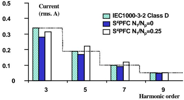
Fig. 6 Harmonic currents of CCM S<sup>4</sup>-PFC with  $N_1/N_p=0$  and  $N_1/N_p=0.25$  at  $V_{in}=230$  V<sub>ac</sub>,  $P_{in}=100$  W and  $V_o=5$  V.
