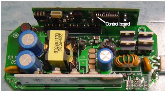
Figure 4. Photograph of the proposed HID lamp ballast.
