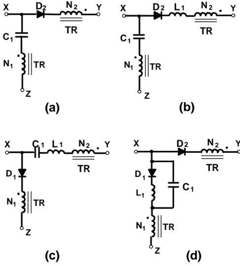
Fig. 6 New implementations of 3-terminal ICS cells (ICS inductor is not shown)
