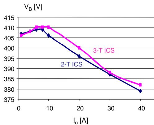
Fig. 19 Bulk-voltage measurements versus load current at maximum line voltage ( $V_{in} = 265 V_{rms}$ )
