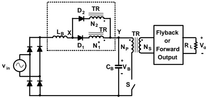
Fig. 10 DCM  $S^2$ ICS circuit with 2-terminal ICS cell corresponding to DCM  $S^2$ ICS circuit with 3-terminal ICS cell Fig. 2
