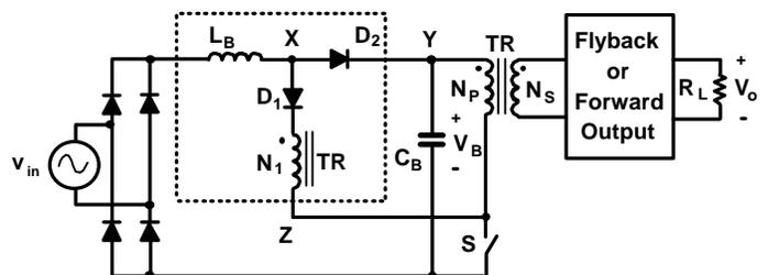
Fig. 1 DCM S<sup>2</sup>ICS circuit with additional winding  $N_1$  [4]
