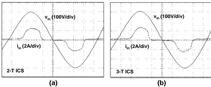
Fig. 16 Experimental line-voltage and line-current waveforms of the  $S^2$ ICS circuit with (a) 2-terminal and (b) 3-terminal ICS cell at nominal line ( $V_{in} = 230 V_{rms}$ ) and full load ( $I_o = 40 A$ )
