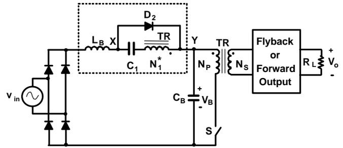
Fig. 13  $S^2$ ICS circuit with 2-terminal capacitive CCM-ICS cell [2]
