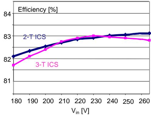
Fig. 18 Efficiency measurements versus line voltage at full load
