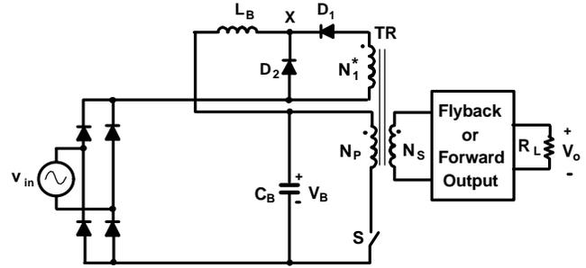
Fig. 8 DCM  $S^2$ ICS circuit with 2-terminal ICS cell [3]
