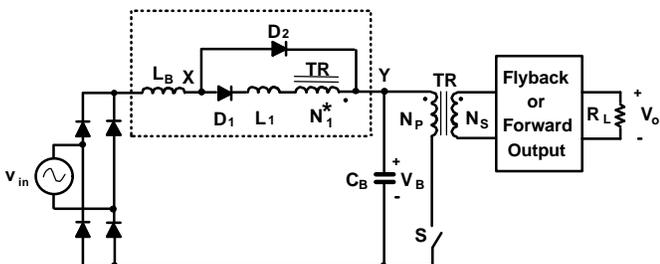
Fig. 12  $S^2$ ICS circuit with 2-terminal inductive CCM-ICS cell [7]
