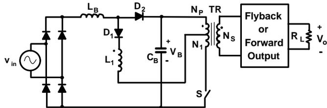
Fig. 7 Implementation of winding  $N_1$  in the 3-terminal ICS cell in Fig. 3 by tapping the primary winding of the power transformer
