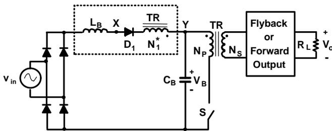
Fig. 11 DCM  $S^2$ ICS circuit with 2-terminal ICS cell (Magnetic switch power supply) [2]
