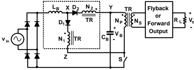
Fig. 2 DCM S<sup>2</sup>ICS circuit with additional windings  $N_1$  and  $N_2$  [5]
