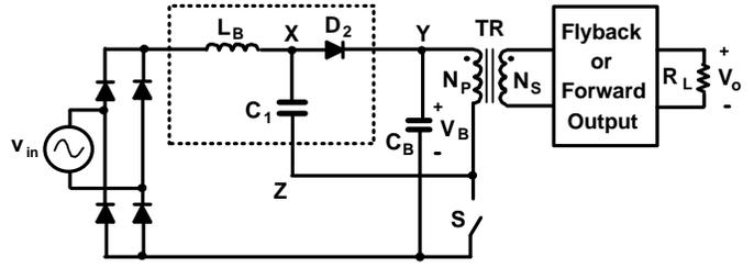
Fig. 4 S<sup>2</sup>ICS circuit with 3-terminal capacitive CCM-ICS cell [1]
