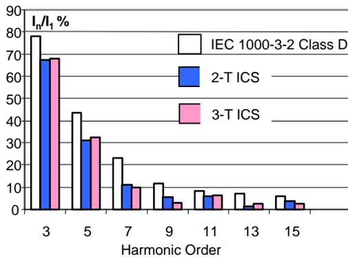
Fig. 17 Experimental line-current harmonics at nominal line ( $V_{in} = 230 V_{rms}$ ) and full load ( $I_o = 40 A$ )
