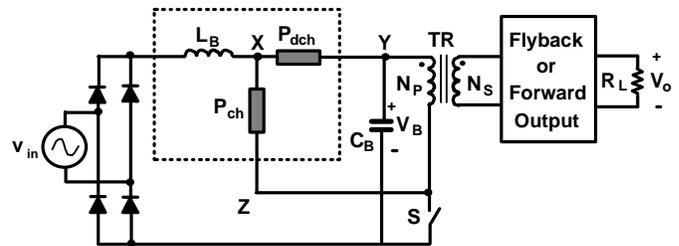
Fig. 5 Generalized topology of S<sup>2</sup>ICS circuit with 3-terminal ICS cell
