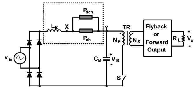
Fig. 14 Generalized topology of  $S^2$ ICS circuit with 2-terminal ICS cell
