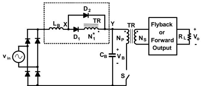
Fig. 9 DCM  $S^2$ ICS circuit with 2-terminal ICS cell in Fig. 8 redrawn
