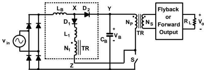
Fig. 3 S<sup>2</sup>ICS circuit with 3-terminal inductive CCM-ICS cell [6], [8], [9]
