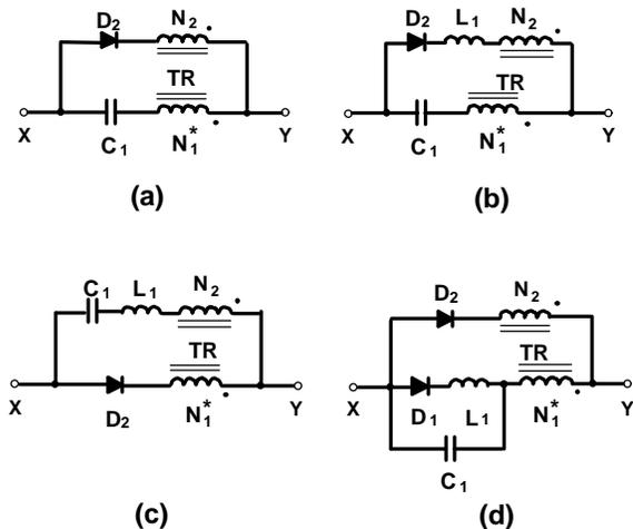
Fig. 15 New implementations of 2-terminal ICS cells (ICS inductor is not shown)
