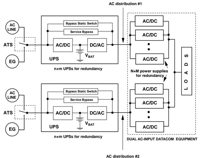
Fig. 2 Dual ac-input power system.
