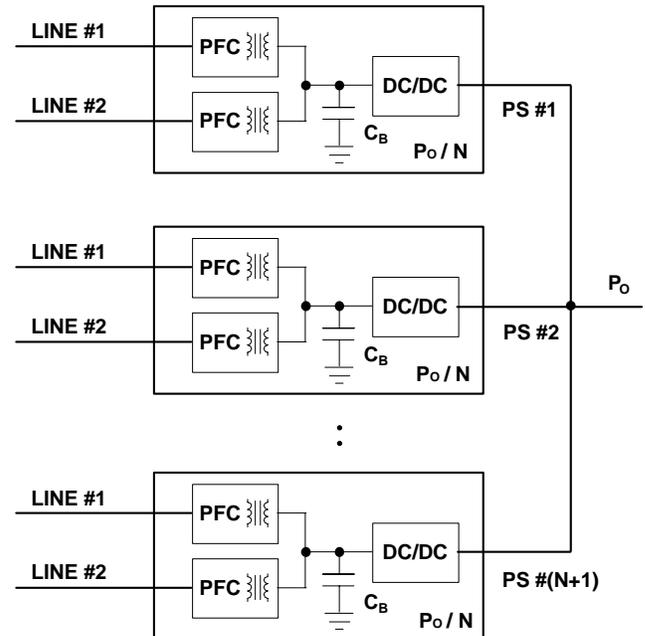
Fig. 5 Dual-Cable-Module Architecture (DCMA).
