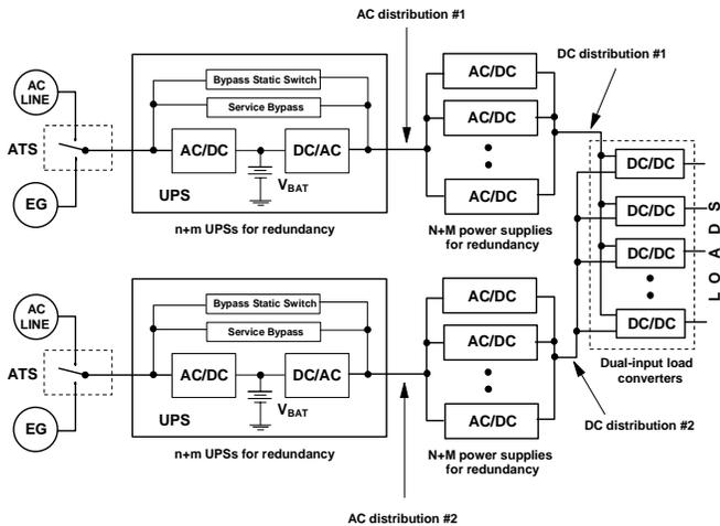
Fig. 3 Power system with dual-input ac/dc and dual-input dc/dc converters.
