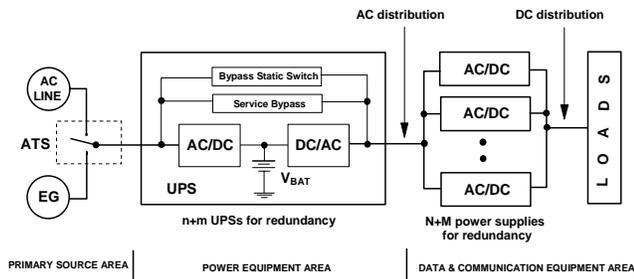
Fig. 1 Typical data center power system.
