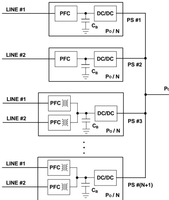
Fig. 6 Mixed Single/Dual-Cable-Module Architecture (MSDCMA).
