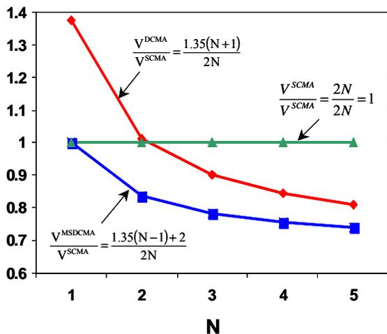
Fig. 7 System power-density comparisons.
