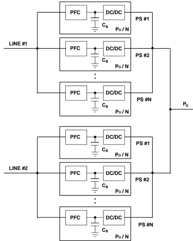
Fig. 4 Single-Cable-Module Architecture (SCMA).
